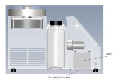
Figure 5: Battery replacement (NT800)
