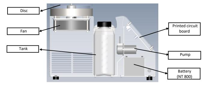
Figure 1: diffuser components
