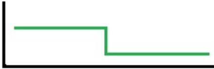
**Green flashing light (1s)** indicates that diffuser is in **starting** phase
