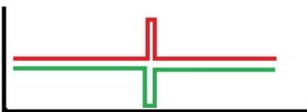
**Green permanent light** associated with a red flash every 2 seconds indicates that dispenser is in diffusion phase and battery charges
